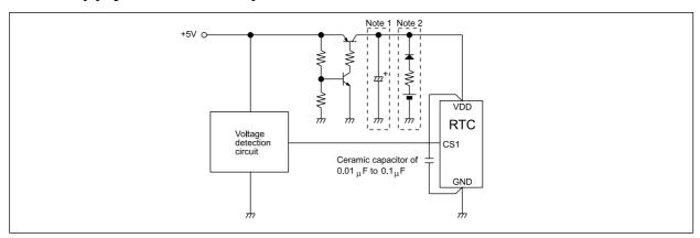
Note 1: This capacitor must be of a high capacity because a transient reverse current flows from the collector to the emitter of the transistor when the power is turned off.
