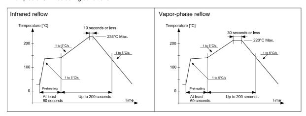
(When increasing the temperature of resin, make sure that these curves are as gentle as possible.)
