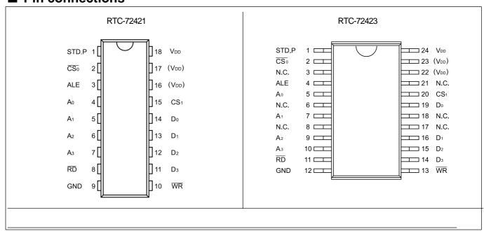
The (VDD) pins are at the same electrical level as VDD. Do not connect these pins externally.
